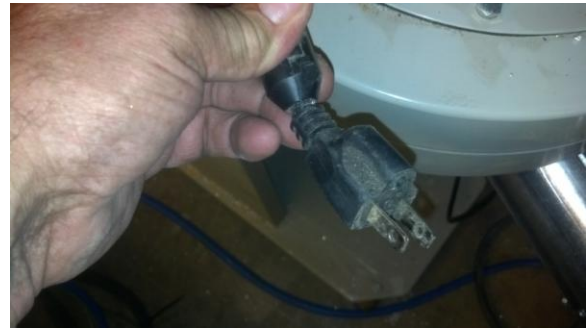
Missing ground lug on dust collector plug (requires adding additional ground wire)
