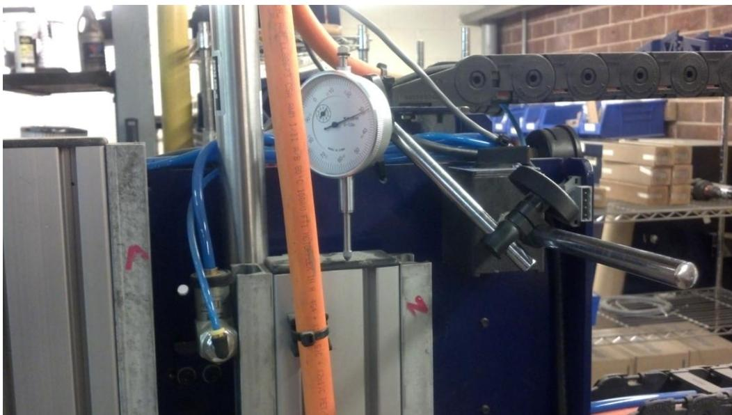
The following are two setups that have the base attached to a table leg and the indicator is touching an upside down 1/2" bit to measure deflection at the bit in the X and Y directions. Push/Pull on the bit or collet nut directly at and away from the indicator.
