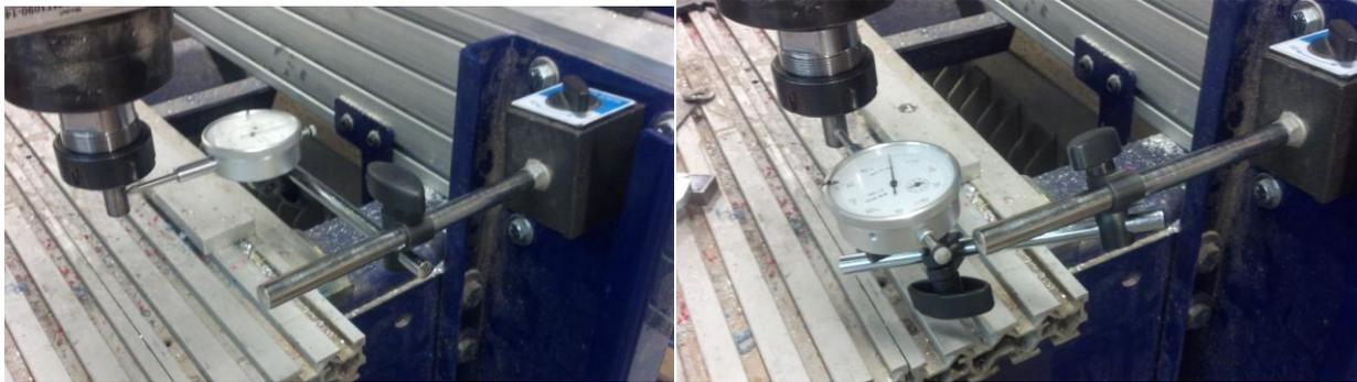
The first 3 setups are directly aimed at the pinion/rack adjustment. The last two, which will show lateral deflection at the bit, can show, depending on the direction, play in the lower YZ car bearings, play in the Z bearings or a loose spindle connections. To gain an accurate assesment at the bit, all play must be removed in the first 3 tests prior to setting up for the last 2.
