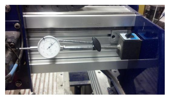
This setup is used to measure play in the Z axis in the vertical direction. The base is attached to the YZ car and the indicator touches the top of the Z extrusion. Grab the spindle or Z extrusion and Push/Pull in the Z (vertical) direction.
