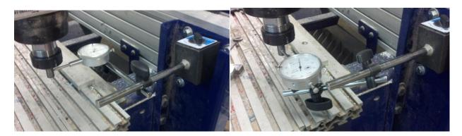
The first 3 setups are directly aimed at the pinion/rack adjustment. The last two, which will show lateral deflection at the bit, can show, depending on the direction, play in the lower YZ car bearings, play in the Z bearings or a loose spindle connections. To gain an accurate assessment at the bit, all play must be removed in the first 3 tests prior to setting up for the last 2.
