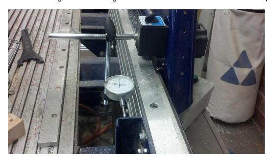
Picture of a Y axis setup with the indicator base attached to a side plate and the indicator against the Y motor. Push/Pull on the YZ car in the Y direction.
