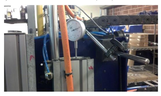
The following are two setups that have the base attached to a table leg and the indicator is touching an upside down 1/2" bit to measure deflection at the bit in the X and Y directions. Push/Pull on the bit or collet nut directly at and away from the indicator.
